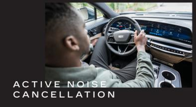
The LYRIQ's sense of quiet luxury is enabled by a suite of noise cancellation technologies. The LYRIQ's enhanced Active Noise Cancellation features take data from the vehicle's accelerometer sensors in each wheel, allowing it to calibrate noise cancellation to create a peaceful, relaxing cabin for our customers.
